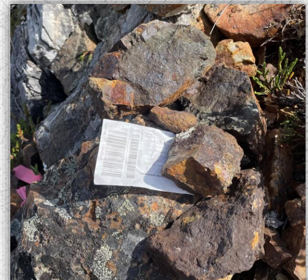
MINERALIZED SKARN HORIZON GRADING 14.1 G/T AU AND 0.43% CU.
