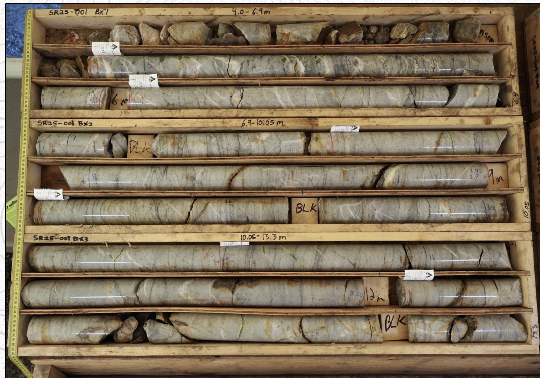
TOP OF FIRST HOLE AT STAR RIVER IN QUARTZITE UNIT WITH PERVASIVE PYRITE-ARSENOPYRITE-GALENA VEINLETS.
