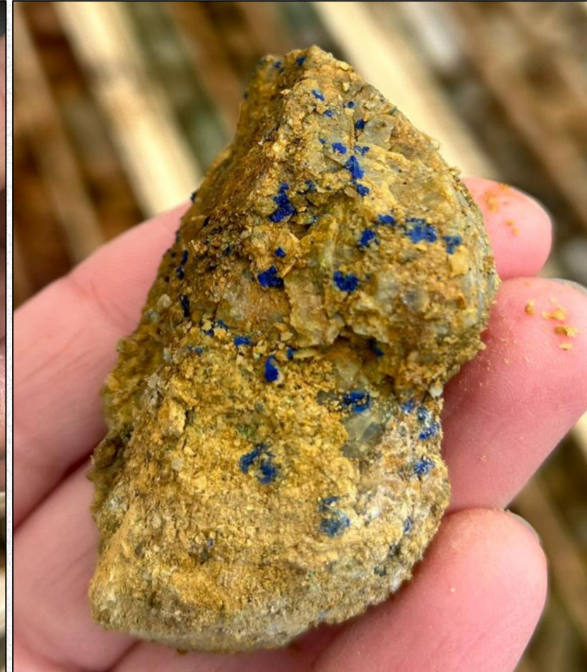
HOLE AZ25-001 AT 13.4M HIGHLIGHTING STRONGLY OXIDIZED CORE WITH ABUNDANT AZURITE MINERALIZATION.
