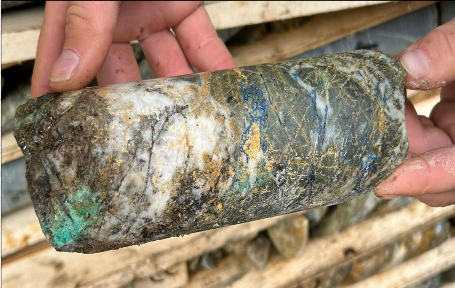
HOLE AZ25-001 AT 22.4M CONTAINING MALACHITE, AZURITE, AND PYRITE.
