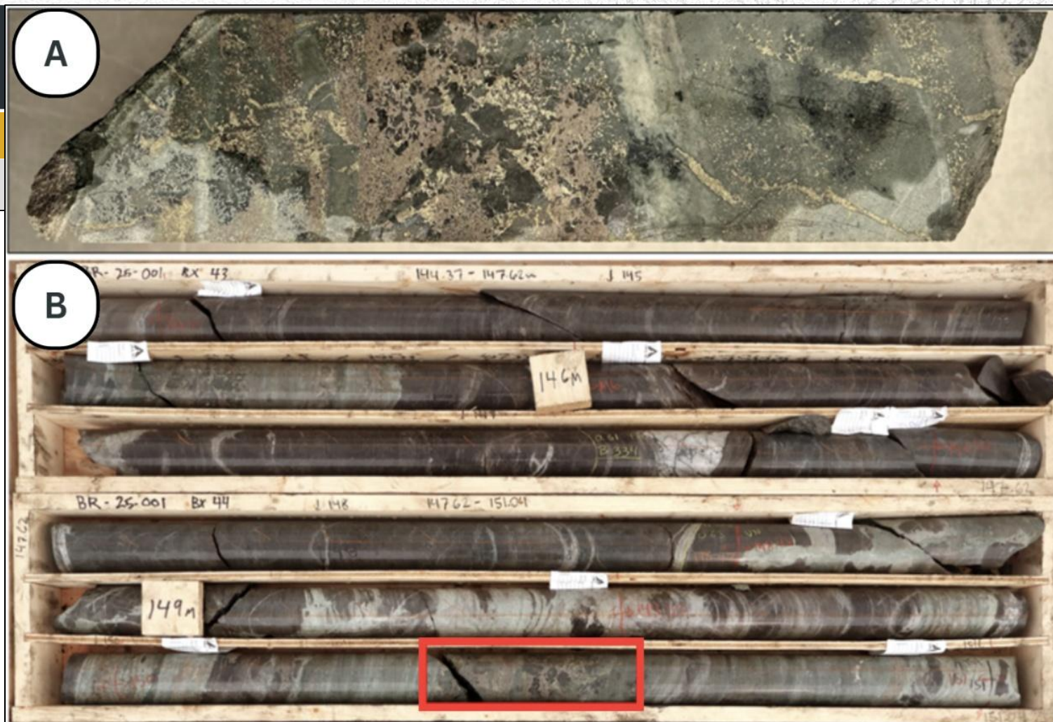
HOLE BR25-001 AT 149M. (A) CLOSEUP OF MASSIVE PYRRHOTITE > CHALCOPYRITE WITHIN SKARN HORIZON. (B) MINERALIZATION WITHIN THE SKARN UNIT CONSISTS OF ZONES OF MASSIVE SULPHIDES AS WELL AS LESS INTENSE FOLIAFORM CHALCOPYRITE.
